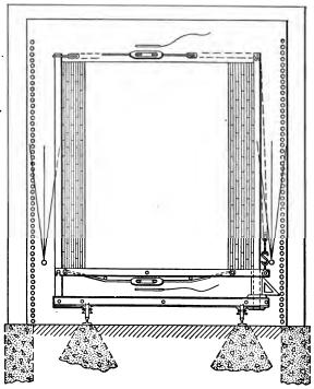
Fig. 97.—Cross section of a compartment kiln operating with superheated steam. Edge stacking with a device for taking up shrinkage is shown. Heating coils are located on each side of the kiln. Steam is admitted between the pile and the coils. The circulation is down through the pile and up on each side. The temperature and quality of steam and the temperature of the heating coils can be regulated to obtain the proper conditions for drying.
